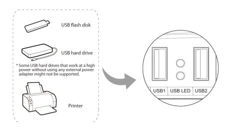
Figure 2-2 USB Installation
